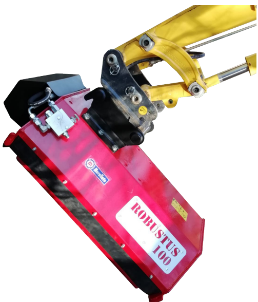
Fig. 2 Testata trinciante pesante ROBUSTUS 120 Heavy duty shredding head ROBUSTUS 120
