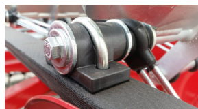
Fig. 3 Dettaglio supportino e boccole in materiale autolubrificante Belt with double-rod connecting bars detail in auto-lubricating material
